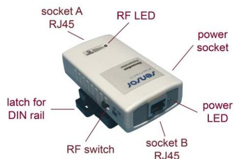
transmission, the socket A enables optional wired connection of the transmitter with wire-less receiver. To do this, move RF switch to the Off position, the RF led is not lit. The transmitter is equipped with a latch for mounting it in a DIN rail.
